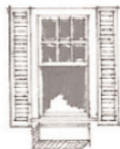
N Shutters too narrow Lower box too narrow
