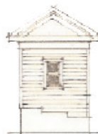
N Inappropriate stepped foundation
