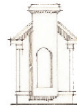
N Cantilever not traditional Inappropriate niche Lack of taper
