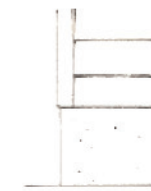
N Siding too wide Cornerboard too narrow
