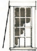
Casing Resembles Post & Lintel
